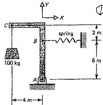
2. For the beam shown in in the right find the reactions  $A_x$ ,  $A_y$  and  $B_y$  at the supports. (12%)
